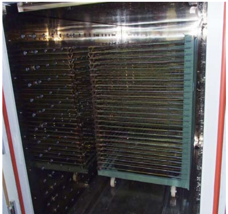
Oven used to heat glass after being printed on with a UV printer at a sign business in Seoul, Korea. At right you see the rack to put several pieces at the same time.
