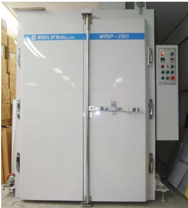
Oven used to heat glass after being printed on with a UV printer at a sign business in Seoul, Korea. At right you see the rack to put several pieces at the same time.
